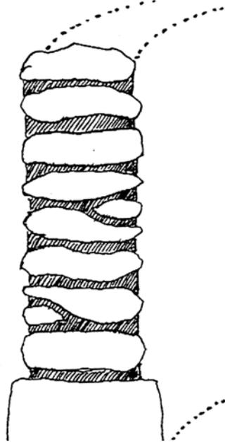
**Figure 4: The foundation layer is wider than the wall**
